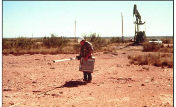
Use of Electromagnetic Conductivity Tool (EM-31) to Delineate Areas of Salt-Impacted Soil Photo courtesy of David Carty
