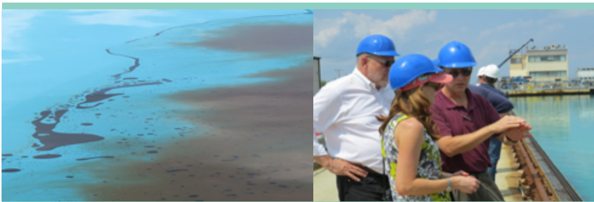
Figure 2. An open house was held at the Ohmsett Facility in July 2014 where attendees observed the effect of dispersants on an oil slick as illustrated by the change in color from black to brown due to the formation of tiny dispersed oil droplets entrained in the water column. (Left) API's Subsea Dispersants Injection Program Chair Tim Nedwed (back center) and Robyn Conmy (front center) of the EPA discuss dispersants chemical behavior while watching on-water demonstrations of dispersants on oil. (Right)
