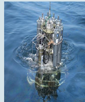
A CTD Rosette, a tool for monitoring water quality, being lowered to collect samples at various depths.
