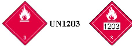
*The illustration showing the UN number to the right of the placard is an example only and does not indicate a mandatory position. For example, a wrap-around label may be used on a cylinder.*
